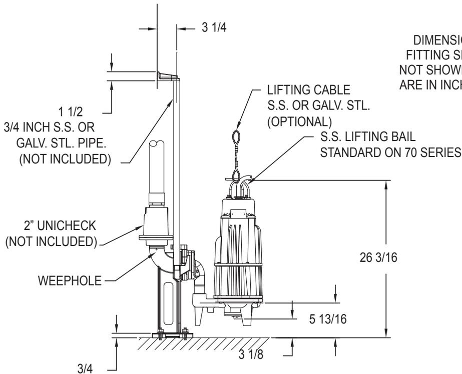
DIMENSIONS ARE BASED ON STD. ANSI FITTING SIZES. CHECK VALVES REQUIRED, NOT SHOWN FOR CLARITY. ALL DIMENSIONS ARE IN INCHES UNLESS OTHERWISE NOTED.
