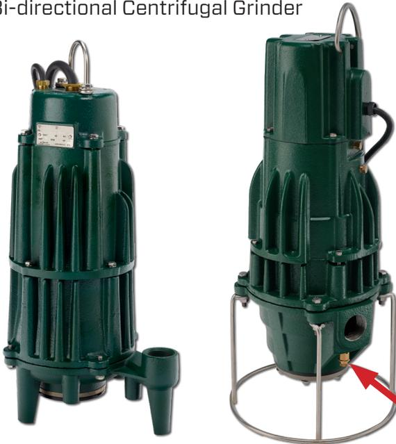
Oil cooled motor and bearings with finned housings. The off position is located above the motor allowing the water in the basin to be used for additional cooling. This design feature promotes longer life. This is a unique feature of the 2 HP oil-cooled progressing cavity grinder pump. Special design features including mechanical seal, rotor, stator, Tri-Slice® cutter, relief valve, and oil filled motor and bearings encourage and deliver long service life.
