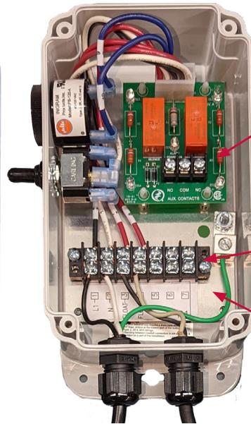
Auxiliary output (dry contacts) for connection to additional alarm equipment, security system, building automation, or input of Z Control® device. 5 amps max, 120 VAC.
