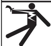
**Hazardous voltage. Can shock, burn or cause death.** Ground pump before connecting to power supply.
