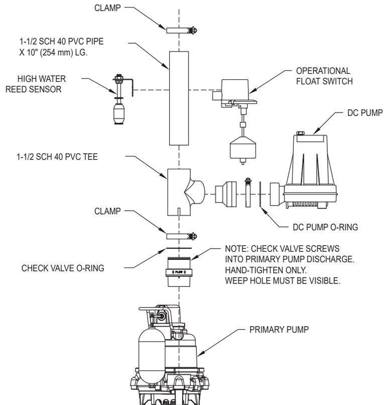
**▲ IMPORTANT** To minimize risk of air lock, intake of DC pump must be set above intake of primary pump.
