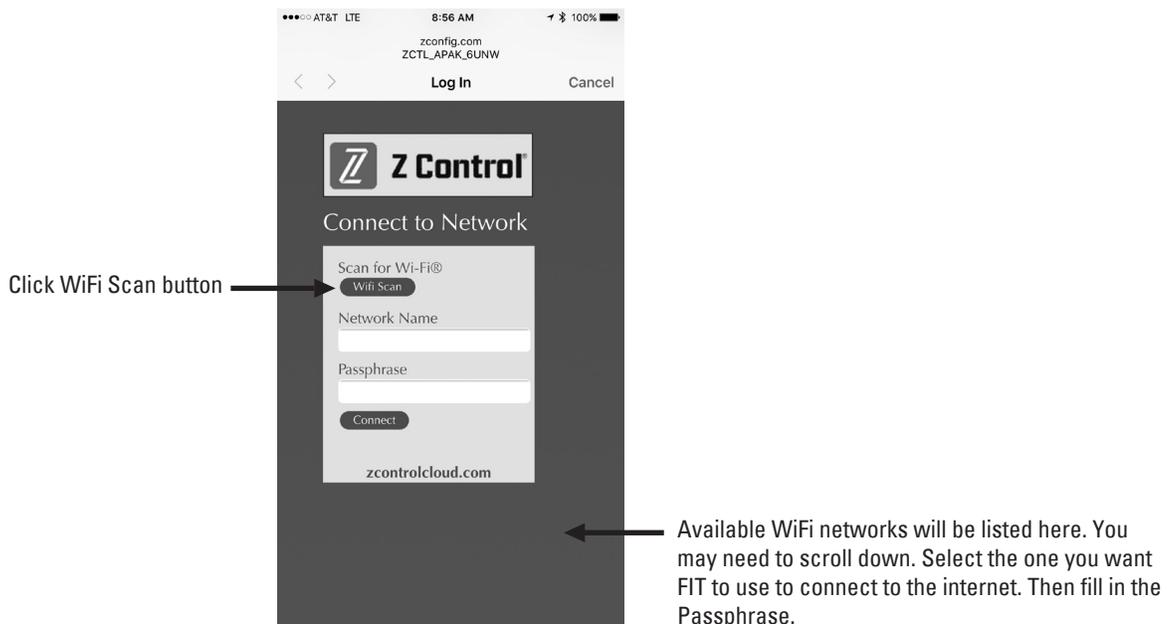
\*\*Note that the Fit will not connect to routers with "WEP" or "OPEN" security. Security must be WPA or WPA2 or similar variant.
