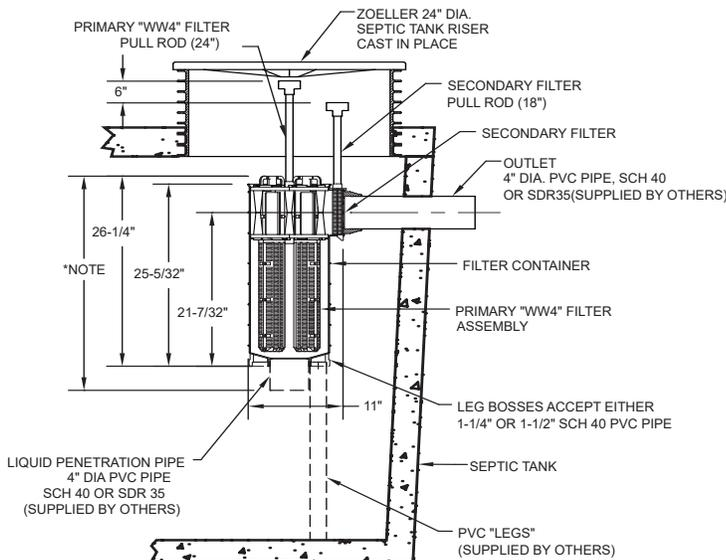
\*NOTE: STATE AND LOCAL PLUMBING CODES MAY REQUIRE A SPECIFIC LIQUID PENETRATION. FOR EXAMPLE, 25% - 40% INTO THE LIQUID DEPTH OR 9" OFF THE TANK BOTTOM.
